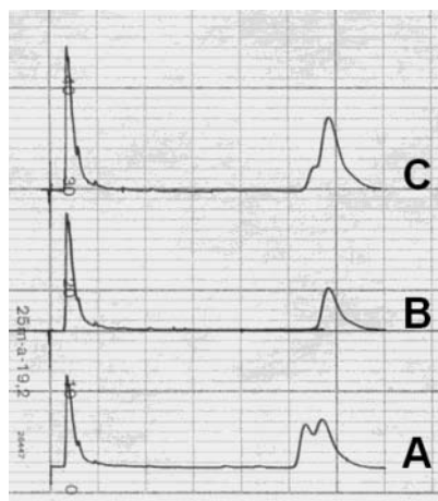
Figure 2. (A) Racemic ( E )-10 (100 \mu L, 1.8 mg/mL). (B) Enantiopure ( R )-( E )-10 (50 \mu L, 1.7 mg/mL). (C) Racemic ( E )-10 (50 \mu L) and enantiopure ( R )-( E )-10 (50 \mu L).
